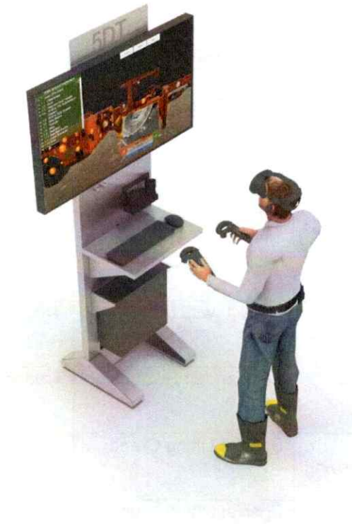
Figure 1 – SimBASE VR Station The user views the virtual world with a virtual reality (VR) head mounted display (HMD). The user navigates in the virtual world and interact with the virtual world with two VR space controllers (wands).
